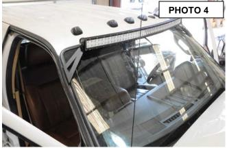
5. With the door shut it may be required to trim the weather stripping so it sits flat on the new brackets.
