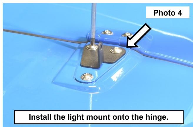
5. Repeat steps 1-4 to install the passenger side light mount onto the vehicle.
