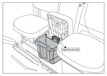
2. Insert integrated handle of storage bin on the seat tube.
