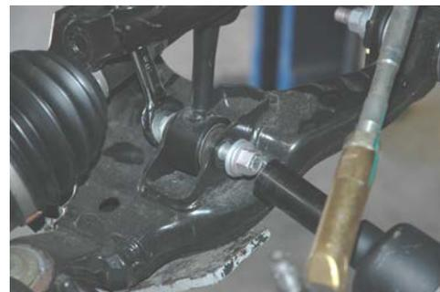
9. Install the new strut extension bracket. Align the holes on the strut extension with the bolts on top of the strut plate and secure with factory hardware. Torque fasteners. **See Photo 7.**
