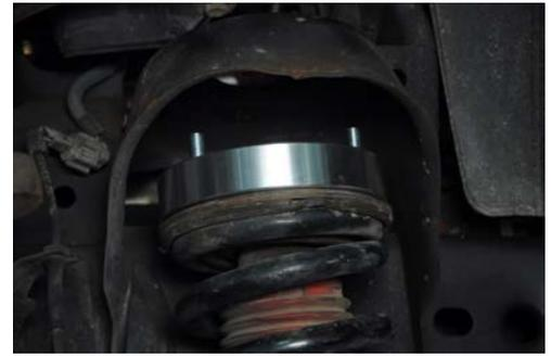
12. Position the strut assembly to reinstall the lower strut bolt in its original position that it was removed. Using original hardware and a 19mm socket torque to 100ft lbs.
