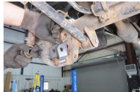
13. Attach shock to bracket using supplied 3/4+bolts, nuts and washers. Tighten using 1 1/16+wrench and 1 1/8-socket. **See Photo 15.**
