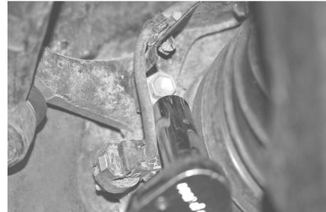
6. Using a 14mm socket, remove the strut nuts on the upper strut tower that holds the assembly in place. **See Photo 4.** One nut can be left on an upper stud to hold the strut in place
