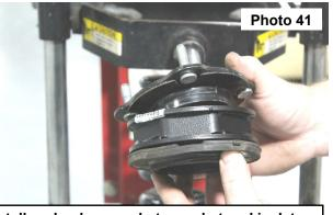
Install preload spacer between hat and isolator.
