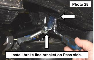
shaft with the stock bolts at the frame and the supplied 5/16" x 3/4" bolts, washer, and nut at the brake lines using 1/2" socket/wrench. See Photo 28, 29, 30, and 31. NOTE: Make sure brake lines do not rub against the top of the frame by bending away from frame slightly.
