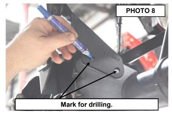
NOTE: For a non 392 model drill the top hole from Photo 9 but for a 392 model, drill the bottom hole.
