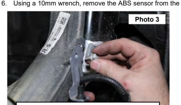
Remove ABS sensor bracket.
