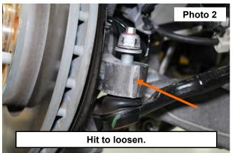
Remove ABS Sensor bracket from knuckle with a 10mm wrench. Retain hardware for reuse. See Photo 3.
