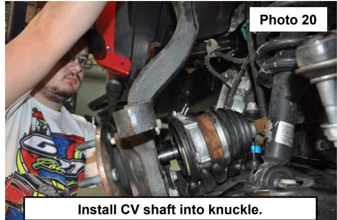
Install CV shaft into knuckle.
