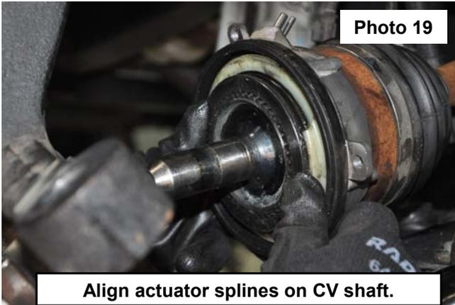
Align actuator splines on CV shaft.
