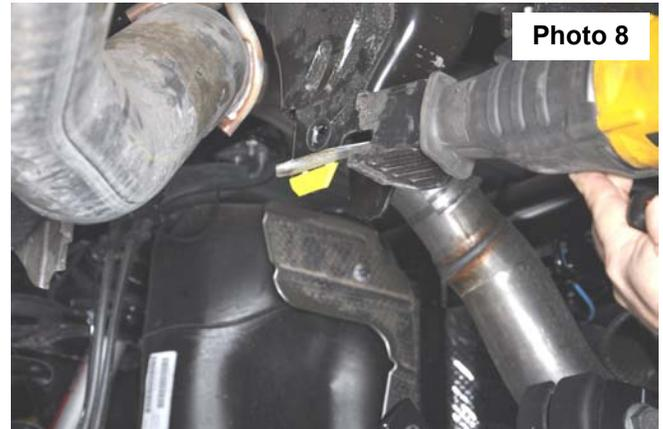
15. Install the new supplied track bar bracket with the crush sleeve using the supplied 9/16" x 4.0" bolt, washer, and nut. Hand tighten. Use the bracket has a template and drill the hole using a 17/32" drill bit. Next install the 1/2" x 1.25" bolt and nut in the drilled hole. Torque the 9/16" bolt to 130ft/lbs with a 13/16" socket & wrench and torque the 1/2" bolt to 90ft/lbs with a 3/4" socket and wrench. **See Photo 9**.
