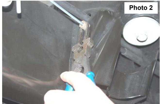
5. Remove the cable and place the supplied drilling template in place, making sure the template has the new hole placed directly below factory hole. The template may be tapped in place.
