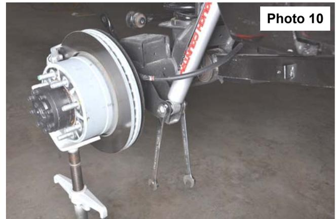
17. Next install the rear sway bar links using the supplied 12mm x 65mm bolts and flange nuts. Torque to 75ft/lbs with a 18mm and 19mm wrench.
