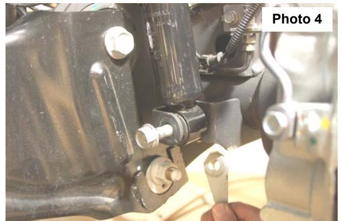
10. Lower the axle and remove the coil springs. Note there is a rubber push pin made on to the factory coil isolator to align the coil spring. Push on the top the pin to release the isolator from the frame coil pocket.
