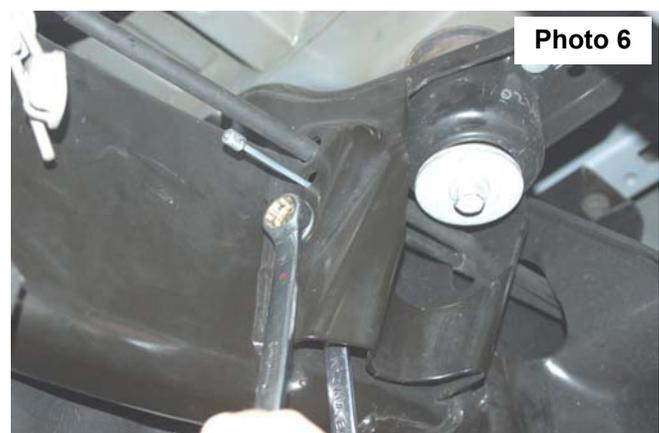
9. Remove the inner fender well using a 8mm socket. 11 bolts to remove. One of the bolts is hidden behind the fender flare on the front side.
