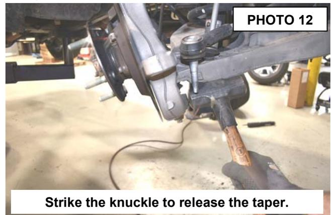
16. Remove the knuckle and retain the stock hardware.
