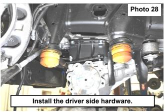
A NOTICE Make sure the differential is pushed to the driver side as far as it can go. Tighten the driver side first using 15mm & 18mm wrenches. Tighten the passenger side using 19mm & 21mm wrenches. Torque to 70 ft-lbs.
