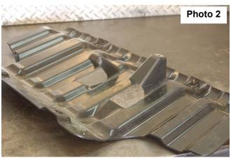
After this area is cut bolt the skid plate back in factory location use the four factory bolts. Tighten with a 15mm socket.
