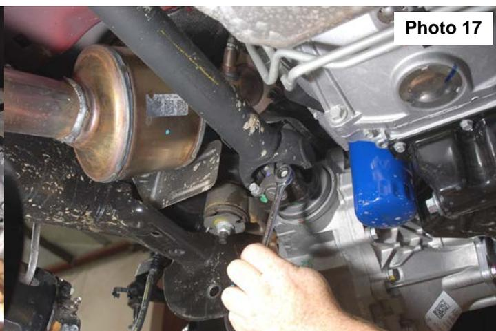
22. Support diff. Using a 18mm socket and 21mm socket remove the bolts from diff. lower diff from truck. **See Photo 18.**
