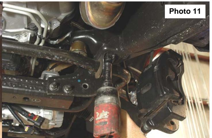
16. Remove the lower control arm using a 18mm wrench and a 24mm socket. **See Photo 12.**
