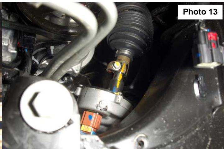
18. Using a 11mm socket, remove the bolt in the intermediate shaft. **See Photo 14.**
