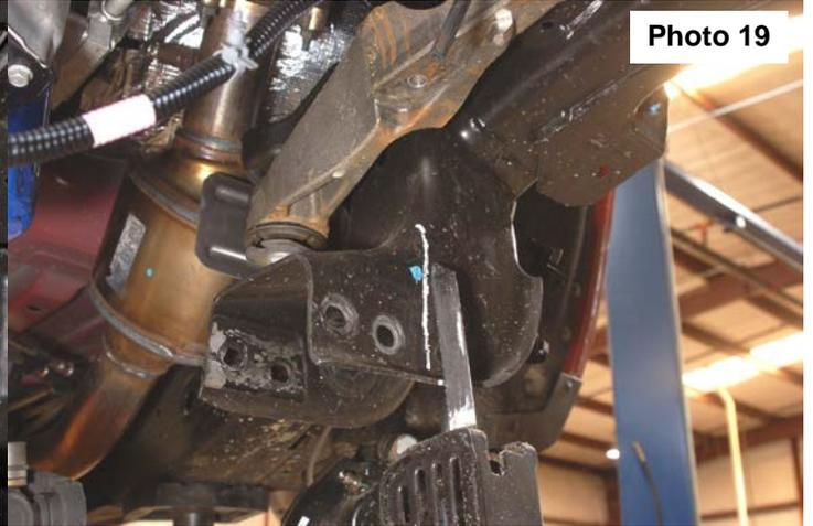
24. Cut and remove the skid plate bracket from the front factory cross-member. Cut the corners out of both front lower control arm pockets. **See Photo 20.**
