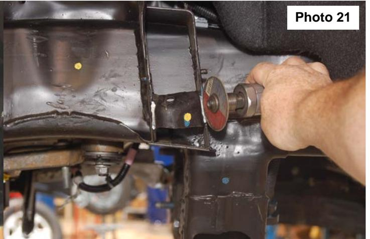
26. Then measure  $1 \frac{5}{8}$ " from the cam bolt pin down and mark both side of the front control arm pocket this is your cut line. Cut straight back to frame then straight down against frame. Clean and paint all cut areas. **See Photo 22.**
