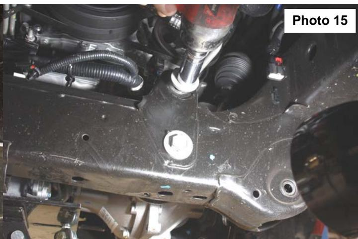
20. Using a 18mm wrench and socket remove the factory lower rear cross-member. **See Photo 16.**
