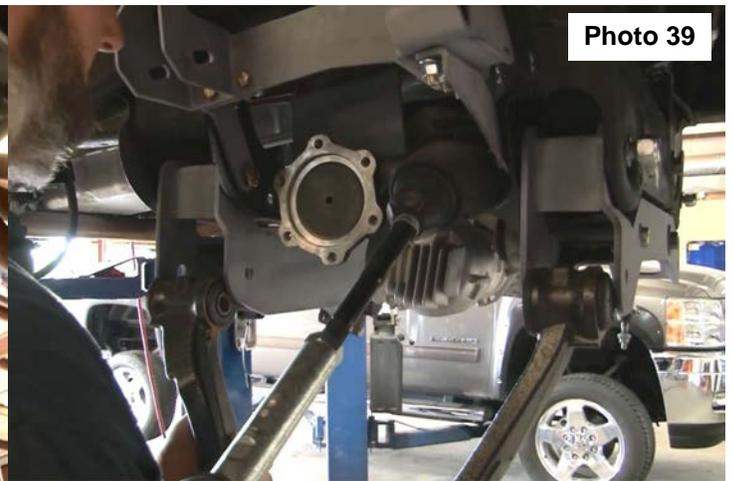
41. Install sway-bar drop bracket using 10mm x 35 mm bolts and washers. Tighten using 17mm wrench. **See Photo 40.** Install sway-bar using stock bolt with new 10mm nuts. **See Photo 41.** Use a 10mm socket and 17mm wrench to tighten. Install stock sway-bar link using a 15mm to tighten.
