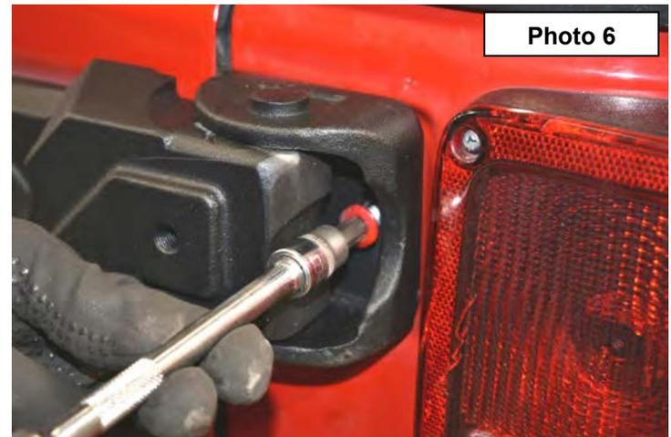
6. Secure the HD carrier to the tailgate using the supplied 8mm x 35mm bolts and washers. Tighten using a 12mm wrench. **See Photo 7.**
