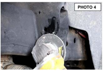
Pull the control arm down out of the way. Insert the bolt and cam washer into the control arm pocket and mark the guide pin so it can be ground flush with the alignment plate. See Photo 2 & 3.
