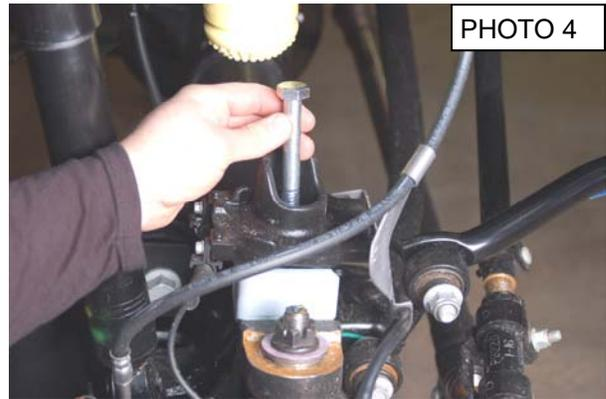
6. Using the floor jack, lower the axle down to allow the coil spring to be removed.
