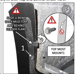
FIGURE G Reinstall factory fasteners through BMF73-LR/RR topmost mount 1, 2, and flap.
