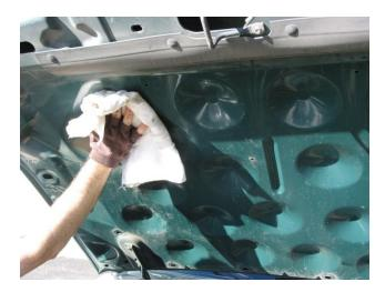
Remove any dust or dirt from the surface of the hood with a dry cloth. With HushMat Hoodliner you don't have to use environmentally unfriendly acetone or alcohol to clean the surface.
