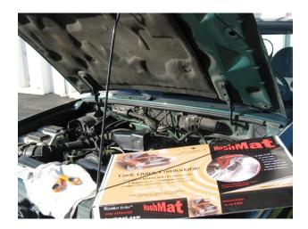
HushMat Hoodliner is formulated to reflect heat away from your hood. The Hoodliner kit contains 12 Square Feet of 1/8<sup>th</sup> inch thick 0.5 pounds per square feet heat reflecting material. This kit is designed to fully treat a full size hood.
