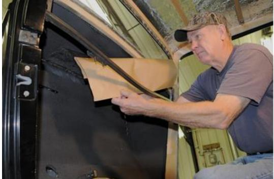
21. The next area to be covered is under the dash/cowl on a '32 Ford. The underside of the cowl is exposed to the outside, so heat and sound deadening is important. This first sheet was placed in the very center under the cowl.
