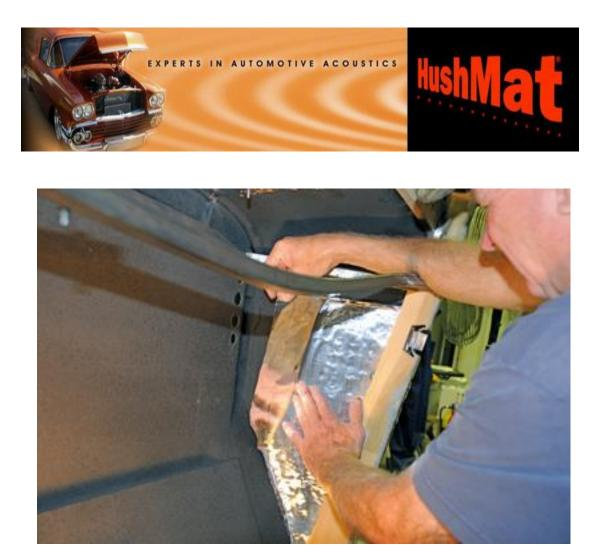
23. The front kick panel area on the passenger side is installed after making a pattern as described earlier.
