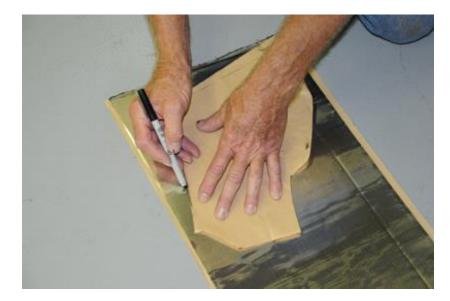
17. After cutting out the drawing made on the backing paper, the pattern is placed on another sheet of HushMat Ultra and traced with a felt tip pen. This process of creating my own patterns allowed me to completely insulate my '32 covering 100% of the surface area.
