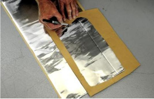
12. Using the template just made, I traced it onto a sheet of HushMat Ultra with a felt tip pen as shown.
