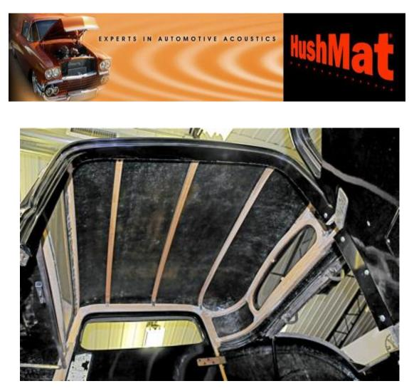
4. The roof in the coupe has wooden bows for attaching a headliner. I unscrewed them from the wood frames around the doors, and removed them for ease of installing the HushMat sheets.
