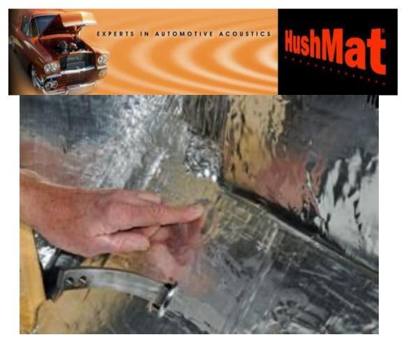
36. The areas to be cut out can be very easily identified by pressing your finger into the depressed areas and then with the utility knife simply cut those areas out.
