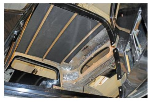
16. The wooden bows were reinstalled after the Silencer Megabond material was installed.
