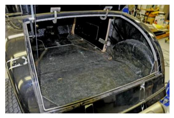
3. The trunk area was open as well so installation was easier. There is no special preparation of the surface needed before installing HushMat. No acetone or other solvent cleaning of the surface was required with HushMat. I vacuumed the complete inside of the body to remove any dirt that was loose on the floor.
