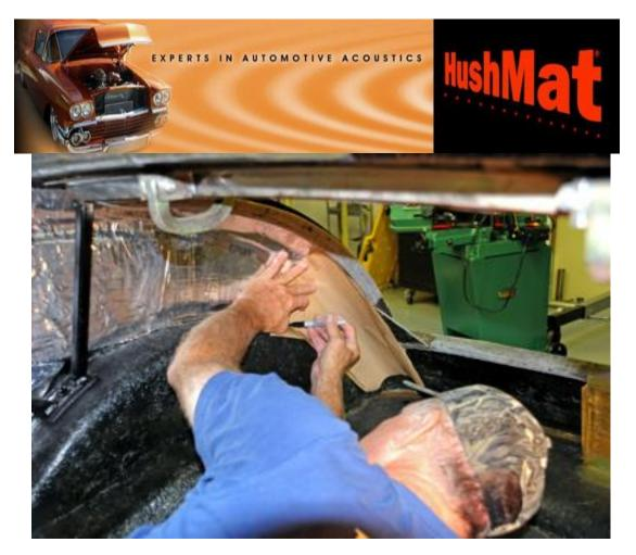
16. The sides of the body were the next area's to cover. The open flat sections were covered first and then patterns were made again using the brown backing paper peeled off of prior sheets. Draw out the area by pressing the paper into the section to be covered and trace it out with a felt tip pen.
