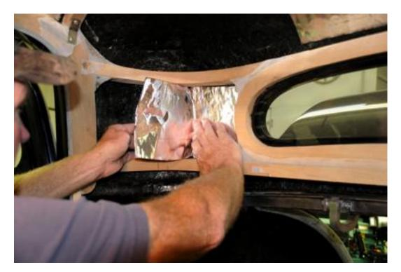
14.The piece of HushMat just cut out can now be easily placed into the tight area next to the rear window as shown.
