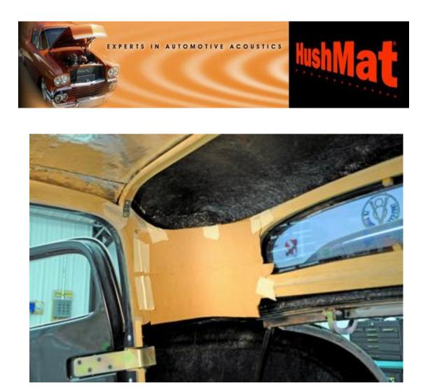
10. The wood frame areas on both sides of the rear window were going to be a problem, so I used a scrap piece of soft cardboard that conformed to the opening. I then used masking tape to hold it in place over the opening.
