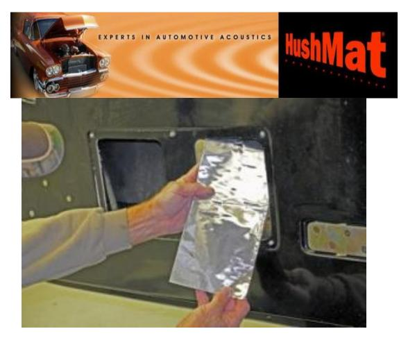
35. I was able to cover almost every square inch inside the doors. The top most areas were covered by using vertical cut sheets as they will reach up to the top of the door easily. This method worked out great!
