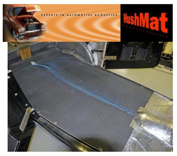
28. The center of the floor was determined next and a chalk line was snapped to mark it.
