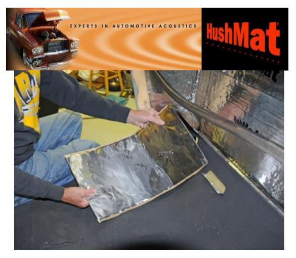
26. The floor is next. The brake pedal arm comes through the floor as most street rods do, so I simply measured where I needed to cut out for it and then slipped the sheet over the pedal arm as shown.
