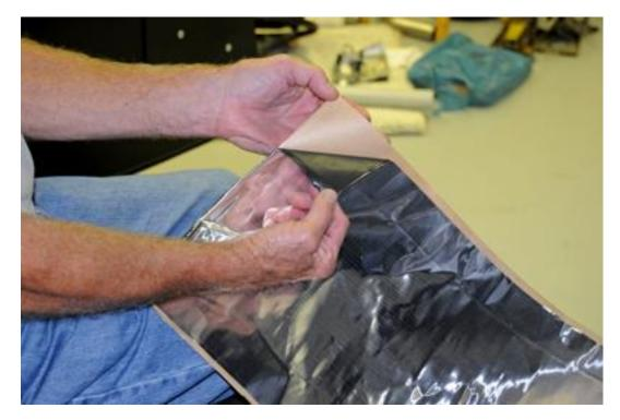
8. You simply peel the brown backing paper off of the HushMat Ultra sheets as shown here. The sheets adhere very nicely to the surface. A good idea is to think ahead of the process and trial fit the pieces before peeling the backing paper off and pressing into place.
