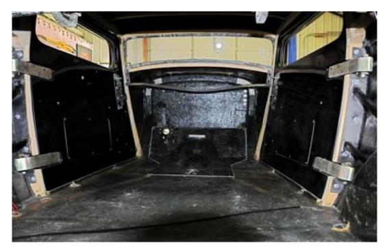
2. This is the bare interior of the 32 Ford coupe fiberglass car body before the installation began. The seat was removed along with the dash, steering column and everything under the dash as this is a new build street rod.
