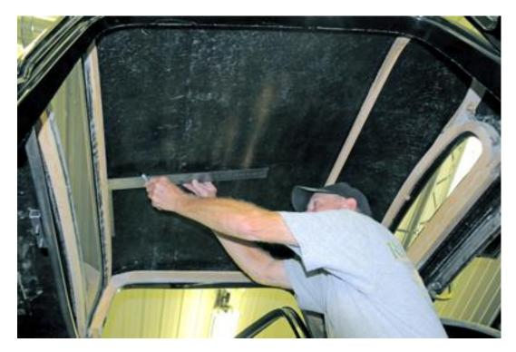
6. After locating the center of the roof area, a straight edge and felt tip pen were used to draw a line on the roof. I found this to be a good way to decide how I was going to install the HushMat Ultra sheets and get the most material use without waste. The HushMat Ultra sheets used are 12X23 inches (which made them very easy to handle and install).
