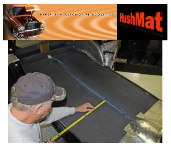
29. Now measure from the center line to determine where the sheets will go to make the best use of all the material and have a neat looking installation.
