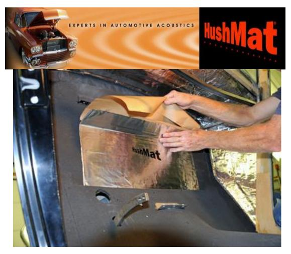
25. The next area to cover is the firewall. Again I started in the center of the firewall and filled in the sides as needed. Simply mark, press, and peel, it's that easy!
