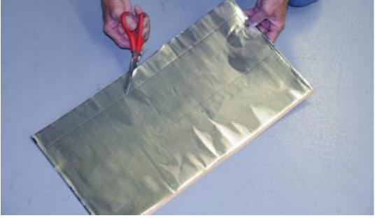
13.Now simply cut out the traced line on the HushMat Ultra sheet using the scissors.
