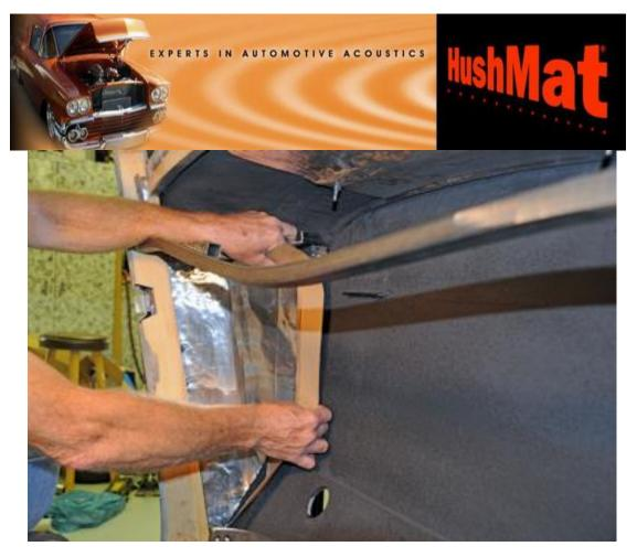
24. Using the same pattern, I merely turned it over or reversed the pattern, to make the piece for the driver side.
