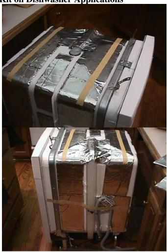
Step 5. Reinstall the insulation pad.
