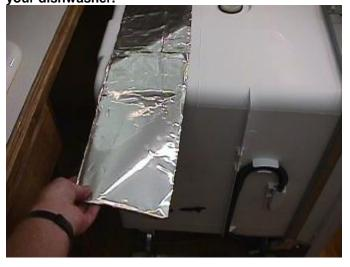
Step 4. After installation of the Ultra pads. Use Hushmat Quiet tape to reattach the insulation pad to the dishwasher as shown.
