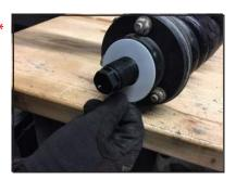
**STEP 15: IMPORTANT!** Be sure the Threaded Adjustment Screw Rotates FREELY after securing kit to the OEM strut. If not, slightly loosen the three upper stud nuts and rotate the Threaded Adjustment Screw slightly **UPWARD**. Re-torque upper stud nuts to OEM specifications and recheck that the Threaded Adjustment Screw now rotates properly for adjustment after installation. If this is skipped the kit will not adjust after installation!!
