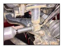
**STEP 10:** Loosen and remove three upper strut mounting nuts.
