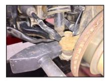
**STEP 8:** Remove upper ball joint cotter pin. Loosen but don't completely remove the nut. Leave it on to protect the threads, but loose enough to remove with your fingers. Use hammer or joint removal tool to separate the taper.
