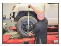
**STEP 27:** IMPORTANT! ADJUSTING FRONT RIDE HEIGHT AFTER INSTALLATION.
