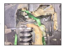
**STEP 22:** Reinstall ball joint nut and torque to manufacturer's specifications. Install new cotter pin (not included).
