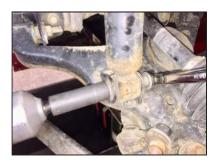
**STEP 21:** Supporting the lower control arm with a jack, use a ratchet strap or similar device to hold upper arm down so ball joint taper seats into knuckle.
