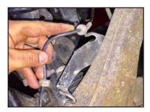
**STEP 6:** Disconnect sway bar from the sway bar link at the top on both sides. Move sway bar out of the way.
