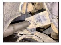
**STEP 17:** Install Top Connection Plate using supplied M10-1.5 nylock nuts. Torque to 45 ft-lbs.
