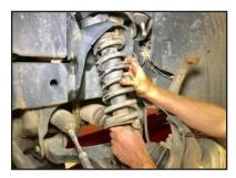
STEP 12: Secure new LIFTmachine kit to the strut assembly, using new M10-1.5 nylock nuts supplied.
