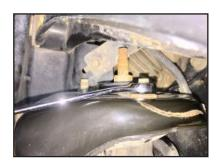
**STEP 11:** Carefully swing knuckle assembly out of the way, taking care to not over extend axle. Slowly lower jack set in Step 4. Remove strut assembly.
