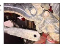
**STEP 7:** Remove tie rod end cotter pin. Loosen but don't complety remove the nut. Leave it on to protect the threads, but loose enough to remove with your fingers. Use hammer or joint removal tool to separate the taper.
