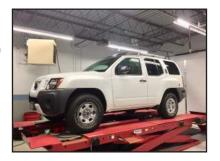
**STEP 26:** Lower the vehicle, jounce suspension and measure ride height of EACH SIDE of the vehicle. Measure from the bottom of the wheel/rim to the lip of the fender.
