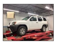
**STEP 2:** On a flat, level surface, MEASURE preinstallation ride height, FRONT & REAR, and write down measurements.
