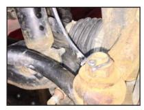
**STEP 24:** Reconnect ABS/Vacuum line brackets, that were disconnected in Step 5.
