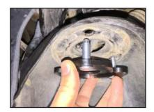
**STEP 18:** Rotate strut assembly 180\* and install into vehicle.
