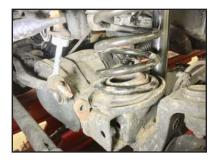
**STEP 5:** Supporting the front axle with suitable jack, disconnect lower shock bolt. Save OEM fastener for use in Step 18.
