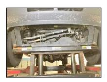
**STEP 4:** Remove sway bar end links. Disconnect ABS/Vacuum lines from bracket to allow slack.
