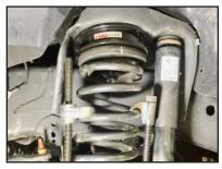
**STEP 17:** Install shock extensions using supplied hardware. Torque to **90** ft/lbs.
