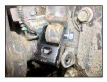
**STEP 18:** Lift axle with jack and rotate extension so nut is on frame side and tighten lower mount with OEM hardware. Torque to OEM Specifications.
