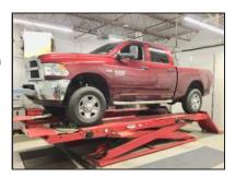
**STEP 25:** Lower the vehicle, jounce suspension and measure ride height of EACH SIDE of the vehicle, front & rear. Measure from the bottom of the wheel/rim to the lip of the fender.
