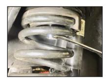
**STEP 23:** Reconnect ABS/Vacuum lines to bracket clips that were disconnected in Step 4.
