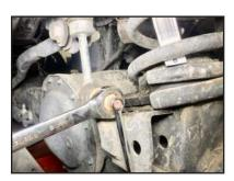
**STEP 20:** To adjust, loosen Jam Nut with 1" wrench one turn. **Do not remove!**
