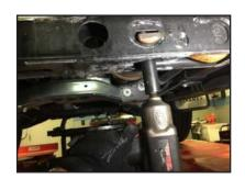
**STEP 10:** Remove both OEM Torsion key Adjusting Bolts.
