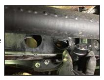
**STEP 16:** Install new Forged 3" 12.9 Adjuster Bolt make sure it has full thread engagement before releasing tension.
