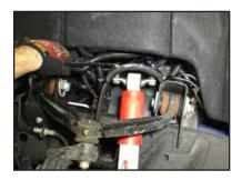
**STEP 8:** Locate the OEM Torsion Keys. They are found where the torsion bars are received into the Crossmember between the frame.
