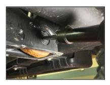
**STEP 13:** Remove OEM Torsion Key. Install ProRyde Torsion Key and slide Torsion Bar back into Torsion Key.
