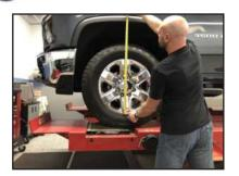
**STEP 3:** Suspend front wheels, lifting by the frame. Secure using jack stands. Make sure wheels are chocked!
