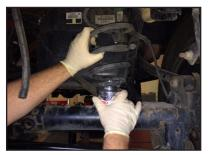
**STEP 12:** Install upper shock extenders, and reinstall shocks using upper hardware, provided, and OE lower shock hardware.
