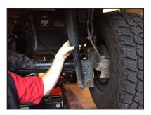
**STEP 7:** Check that all brake lines, hoses & ABS lines have proper slack, disconnecting mounting hardware, as required.
