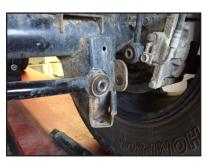
**STEP 6:** Remove rear shocks, and retain hardware for reinstallation.
