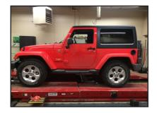
**STEP 2:** Position vehicle on a stable, flat surface or automotive lift.
