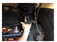
**STEP 16:** Install brake line relocator brackets on each side of vehicle using included hardware, as shown.
