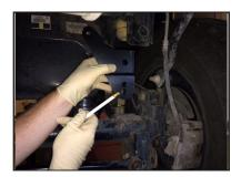
**STEP 15:** Reconnect rear track bar to your chosen anchor point, as shown, and torque to OE specs.
