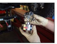
**STEP 10:** Install chosen spacers over bottom rear coil locator, and secure with included hardware, as shown.
