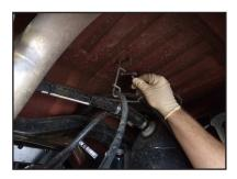
**STEP 3:** Disconnect Sway bar links at each end of sway bar, as shown.
