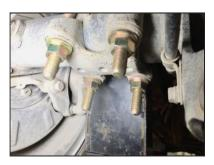
**STEP 11:** Install shock bolt and nut. Torque to manufacturer's specifications.
