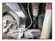
**STEP 10:** Slowly lower vehicle making sure the alignment pin lines up with alignment hole on block. Tighten new ubolts evenly in a crisscross pattern.
