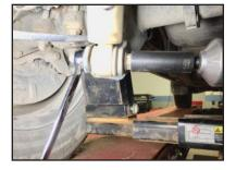
**STEP 5:** Remove the four U-bolt nuts and washers on each side of the vehicle, and remove lower U-bolt axle brackets.
