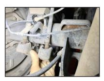
**STEP 6:** Lift vehicle by frame or leaf spring. Remove factory rear block.
