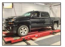
**STEP 2:** On a flat, level surface, MEASURE preinstallation ride height, FRONT & REAR, and write down measurements. Front (L)\_\_\_\_\_\_ Front (R)\_\_\_\_\_\_ Rear (L)\_\_\_\_\_ Rear (R)\_\_\_\_\_\_ Rear (R)\_R RAAR (R)\_R R
