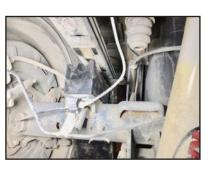
**STEP 8:** Utilize two lower blocks together to get 1.5" rear lift as shown here.
