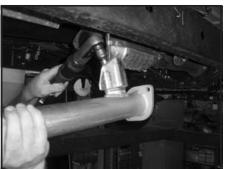
12. Install Oxygen sensor into new intermediate pipe (A) using factory 12mm hardware.
