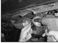
14. Using the 14mm wrench, socket, and ratchet, tighten the Catalytic Converter bolts and nuts.
