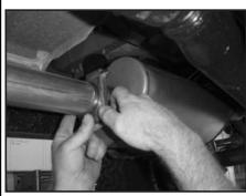
15. Insert intermediate pipe (A) into muffler (B) and install exhaust clamp (D) at the front of the muffler (B).
