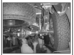
8. Remove factory exhaust from the vehicle.
