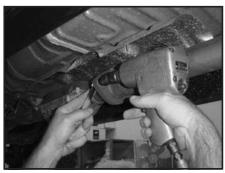
3. With the vehicle raised and properly supported, use the 14mm wrench, 14mm socket and ratchet to remove the bolts from the Catalytic Converter flange.
