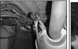
5. Using the pry bar, remove the tail pipe hangers from the rubber isolators.
