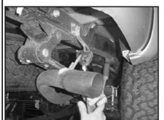
7. Remove tail pipe hanger from factory rubber isolator.
