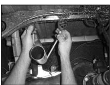
10. Insert front tail pipe hangers into factory rubber isolators.
