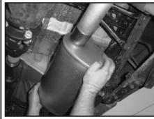
11. Slip muffler (B) into the tail pipe (C) as shown in the photo.
