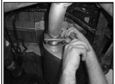
16. Install exhaust clamp (D) at the rear of the muffler (B).
