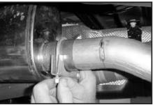
11. Attach clamp (E) to the front of the muffle
