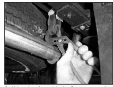
5. Using the channel lock pliers, remove the tail pipe hanger from the rubber isolator.
