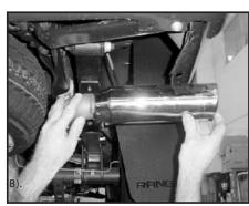
16. Align tail pipe (C). tighten clamp (D).
