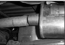
13. Insert tailpipe (C) into muffler (B).
