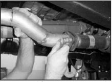
7. Using original fasteners, connect intermediat pipe (A) to the factory catalytic converter pipe.
