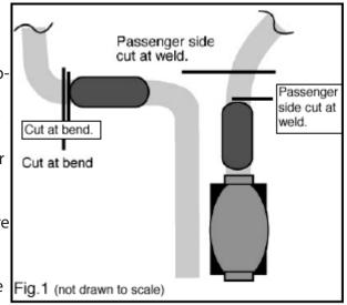
13. You will now need to cut the catalytic converter pipes where indicated (see drawing below).
