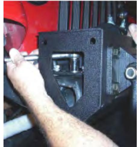
7. Inspect all mounting bolts to make sure they have been tightened. Double check D-rings to make sure they are secured to bumper cover and sub-frame. Reinstall side cover plates to bumper cover. Run winch power leads and make sure they DO NOT rub on XHD bumper cover or sub-frame.
