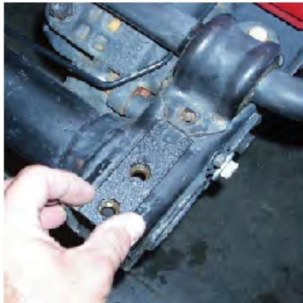
3. Mount winch to sub-frame making sure all lead wires have been connected. Two sets of mounting holes have been supplied for different winch designs. Most applications will use left mounting holes.
