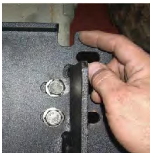
5. For 1987 - 2006 Wranglers, place sub-frame and winch assemble onto vehicle frame with spacers in place (see step 2). Align holes and secure reusing original hardware removed in steps 1 and 2. TJs will use the first, second, and fourth sub-frame mounting holes. YJs will use the first and third sub-frame mounting holes. Snug bolts but **DO NOT TIGHTEN** at this time. Adjustment of sub-frame from side to side will be needed later.
