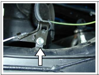
1. Remove bolt securing ABS wire bracket to rear axle housing as shown by arrow.
