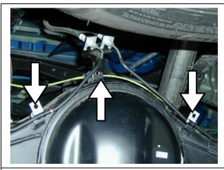
1. Remove bolts securing brake line as shown by arrows.
