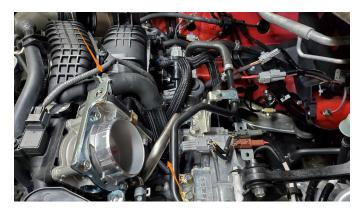
**06.** Using a 10mm socket loosen, but do not remove, the bolt securing the ground strap shown in the photo below.
