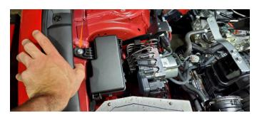
11. Install the straight end of the hose that was assembled in step 3 onto the PCV valve and secure with (1) supplied 20-32mm worm gear clamp. A 7mm socket, swivel adapter, and extensions may be needed to reach the worm gear clamp to tighten.
