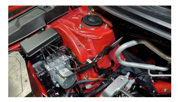
**07.** Using a 10mm socket, remove the bolt shown in the photo below so the electrical box can be pushed slightly out of the way. The rubber engine bay trim may need to be pushed back to access this bolt.
