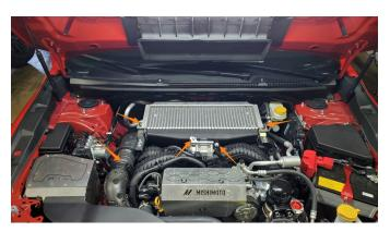
**05.** Remove the OEM PCV to intake manifold hose using pliers to loosen the (2) spring clamps. Long reach needle nose pliers and/or a remote-action hose clamp tool will make this much easier.
