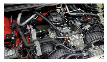
13. Install the hose from the intake manifold, that was just installed in step 12, onto the catch can port labeled "OUT" and secure with [1] supplied 16-25mm worm gear clamp. Then install the hose from the PCV valve, that was installed in step 11, onto the catch can port labeled "IN" and secure with [1] supplied 16-25mm worm gear clamp. (Image on next page)
