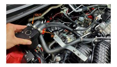
**14.** Using a 4mm allen key, secure the catch can bracket to the mounting bracket with the (2) supplied M6 bolts. These bolts can be removed to get better access to unscrew the catch can bottom for servicing.
