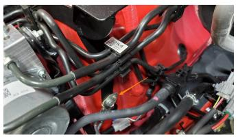
**10**. Using a 10mm socket, reinstall the bolt for the electrical box that was removed in step 7.
