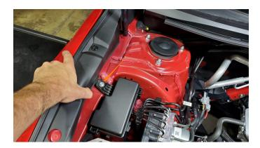
**08.** Using a 12mm socket, remove the bolt from the stud shown in the photo below.
