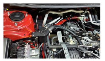
**15.** Reinstall the intercooler by reinstalling the (4) bolts and (1) spring clip that were removed in step 4. Ensure the spring clip is fully seated in the charge pipe coupler. The installation is now complete.
