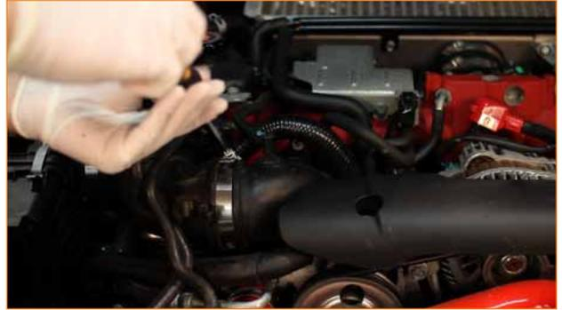
4. Once the clamps are loose, remove the air intake hose from the vehicle.
