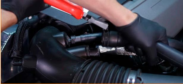
03. If you want to delete your sound generator, loosen the clamp at the other end of the sound-generator hose. Remove the hose by lifting it upward near the clip that secures the hose to the airbox. Follow the sound-generator tube back to the firewall and remove the nut that secures it. Then remove the sound-generator tube and install the provided firewall plug to seal the port. (1x 10mm nut, 1x spring-clamp, 1x worm-gear clamp)
