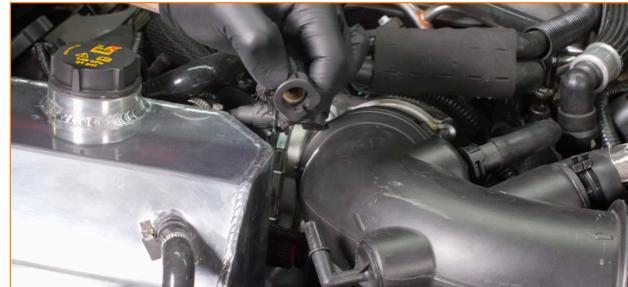
05. Remove the rear hose from the intake pipe using the same process.
