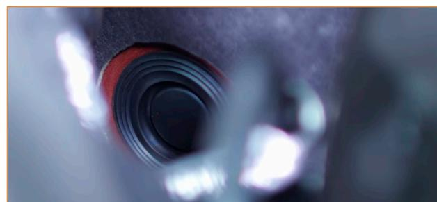
04. Remove the front hose from the intake pipe by depressing the black tab and pulling the hose off the pipe.
