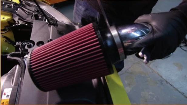
**21.** Attach the upper rubber bushing to the intake pipe. The unused threads must be facing upward. (10mm ratchet wrench)
