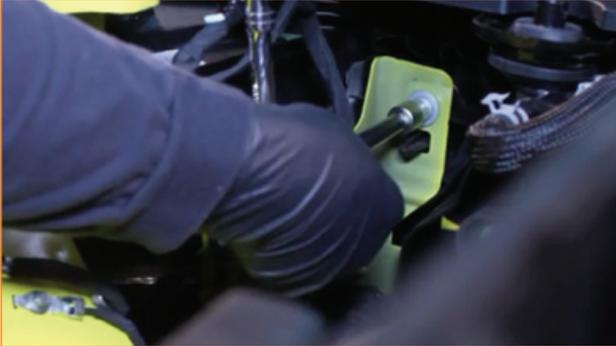
**14.** Remove the tree clips from the harness on the bottom of the wheel well. (flathead screwdriver)
