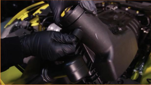
**6.** Remove the spring clip from the bypass valve hose, and remove the bypass valve hose from the stock intake pipe.
