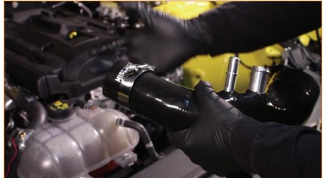
**11.** Reconnect the quick-disconnect fitting. You should hear the plastic tabs snap into place.
