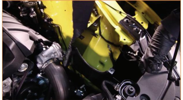
**17.** Make sure that the tab on the airbox falls in line with the ground bolt, and fully tighten the 8mm ground bolt.
