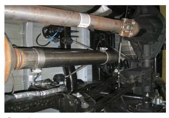
**Step 3.** The longer Inlet Pipe Extension will be needed for Long Bed applications only.
