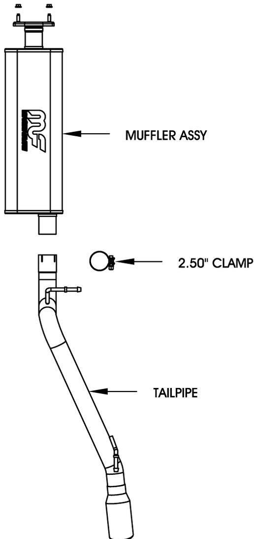
**Step 1:** (Carefully read all instructions before installation.) To begin removal of the OEM exhaust system, unbolt the muffler from catalytic converter extension pipe. Do not discard the OEM fasteners, as they will be re-used on your new system. Remove the muffler and tail pipe from the OEM rubber insulators. Do not damage the rubber insulators, as they will be re-used on your new system.
