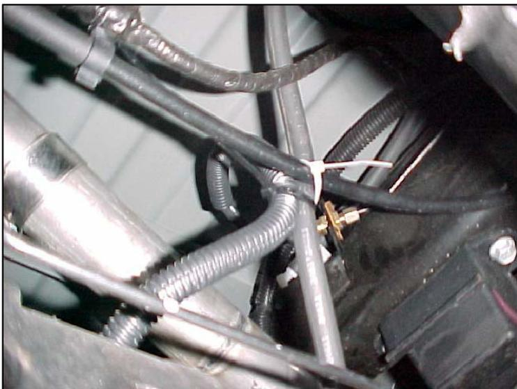
**Step 4:** Once a final position has been chosen for the new system, evenly tighten all fasteners from front to rear. The supplied band clamps must be VERY tight to properly align the pipes and prevent leaks (Approximately 40ft-lbs.) Inspect all fasteners after 25-50 miles of operation and retighten if necessary.
