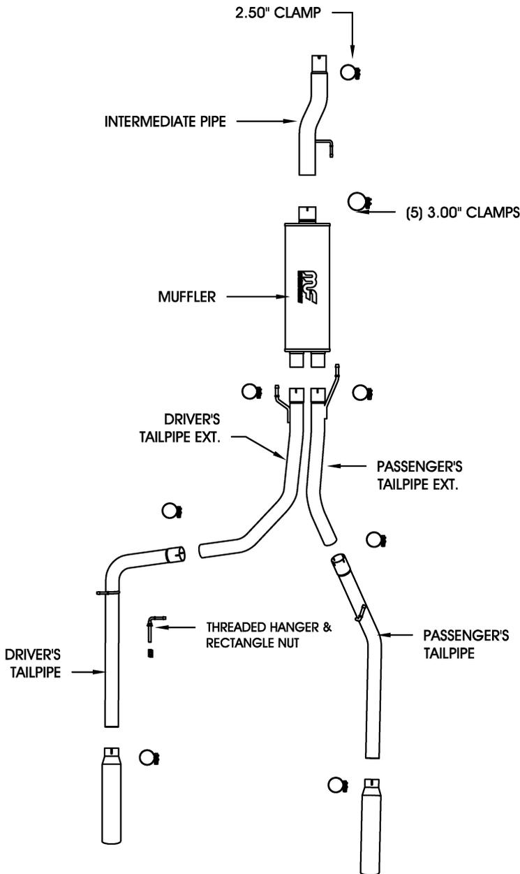
**Step 1:** (Carefully read all instructions before installation) Remove the OEM exhaust system by unbolting the OEM clamps and by disengaging the welded hangers from the OEM rubber insulators. Do not discard the OEM fasteners, or damage the OEM rubber insulators, as they will be reused to mount the new system.
