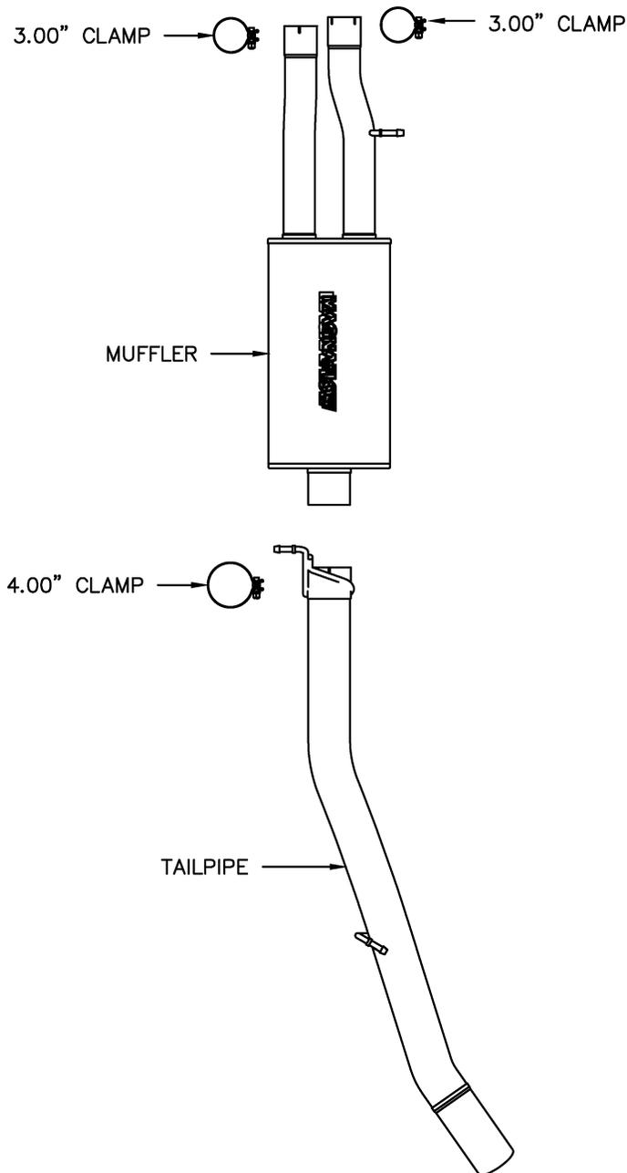
**Step 1:** (Carefully read all instructions before installation) To remove the OEM exhaust system, you will need to cut the exhaust pipes 60" ahead of the center of the rear axle. You may also need to cut the tailpipe about 1" behind the muffler to aid in removal of the system. Do not damage the OEM rubber insulators when removing the OEM system, as they will be re-used to mount the new system.
