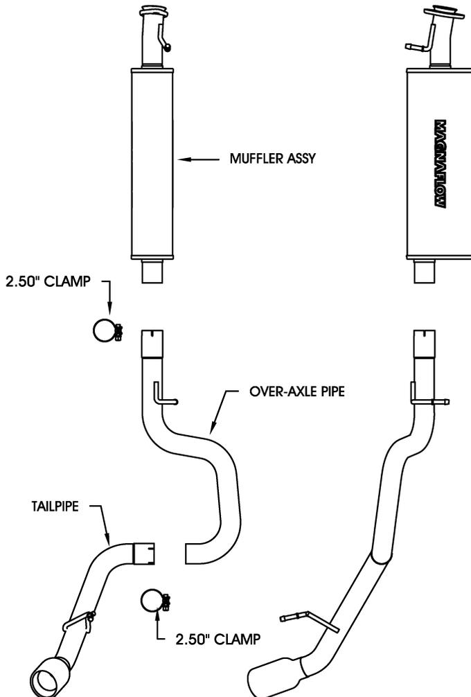
**Step 2:** Begin installation by fitting the welded hanger on the muffler extension pipe into the OEM rubber insulator and fastening it to the catalytic converter at the 2-bolt flange (Leave all clamps and fasteners loose for final adjustment of the complete system). Install the over-axle pipe by fitting the welded hanger into the OEM rubber insulator and by fastening it to the muffler using a supplied 2.50" clamp. Install the tailpipe in a similar fashion.
