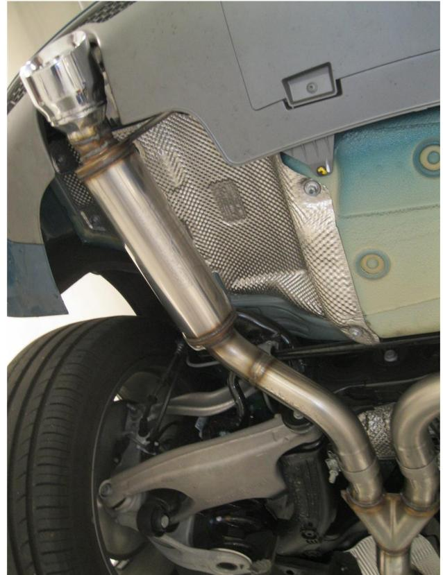
**Step 3.** Then install D/S Muffler Assembly in a similar fashion as the Y-Pipe assembly using the supplied 2.50" clamp and inserting the hanger into the OEM rubber insulators.
