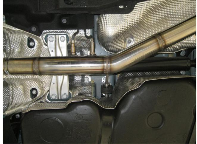
**Step 2.** Begin installation of your new MAGNAFLOW exhaust system by attaching the Y-Pipe Assembly to the resonator outlet using the OEM clamp. Insert the hanger into OEM rubber insulators and re-install the O2 sensors.
