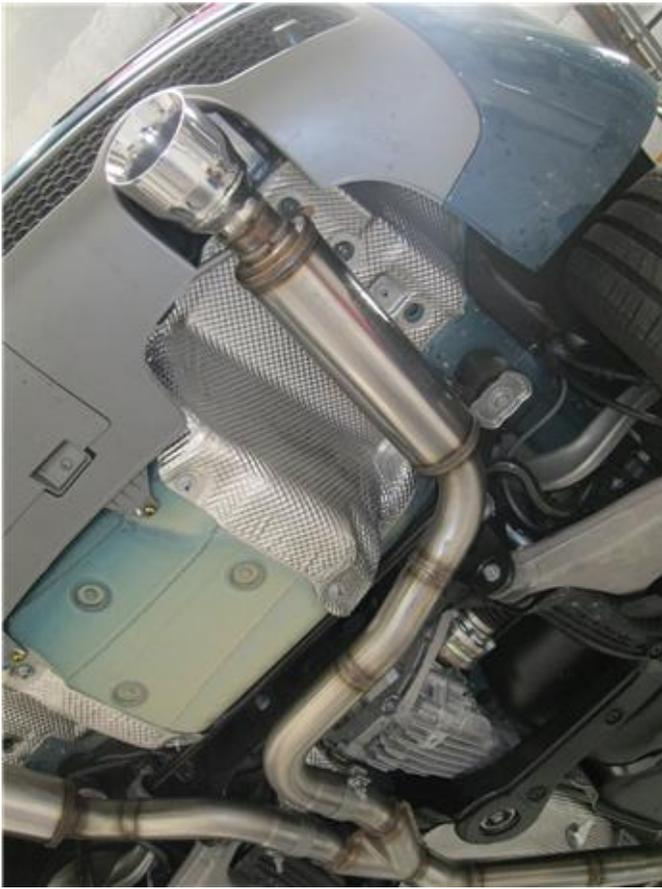
**Step 4.** Next install the P/S Muffler Assembly in similar fashion as the D/S using the supplied 2.50" clamp and inserting the hanger in to the rubber insulator.
