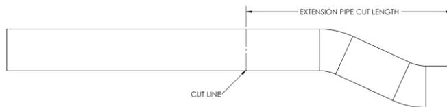
**Installation Tip:** Temporarily install the **Muffler** and the **Over-Axle Pipe** using the factory rubber insulators and the **Dual Hang Tight™ Hanger** assembly. Measure from the **Muffler** to **Adaptor 3.5" to 4"** the and cut the **Extension Pipe** to the required length.
