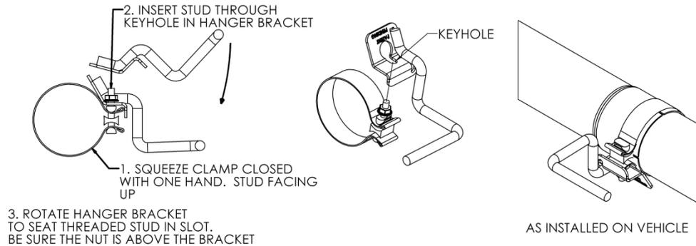
8. Install the front single **Hang Tight™ Hanger** assembly onto the **Extension Pipe** and into the OEM rubber insulator.
