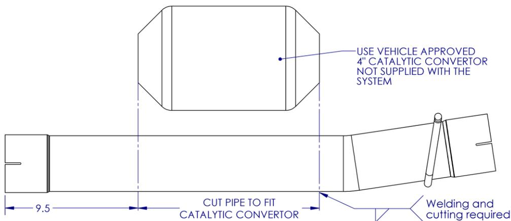
ADAPTOR PIPE TO WORK WITH 4" CATALYTIC CONVERTORS
