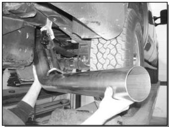
6. Install the **Tail Pipe** from the rear of the truck, over the axle and attach to the **Muffler Outlet**. Install the tail pipe hanger into the OEM hanger, and then adjust for best axle clearance and **Tail Pipe** exit location to complete. **See Figure 10.**
