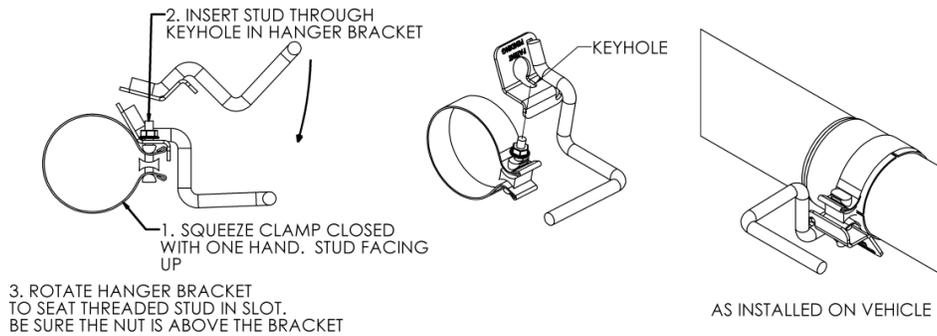
6. Install the appropriate **Hang Tight™ Hanger** over the **Extension pipe** and into the OEM rubber hanger. Install the **Muffler** over the **Extension Pipe** using the next **Hang Tight™ Hanger**. Install the **Dual Hang Tight™ Hanger** into the two OEM rubber hangers located above the outlet of the **Muffler**.
