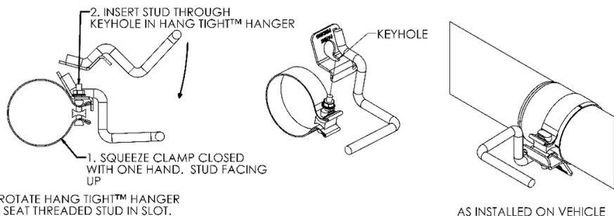
3. ROTATE HANG TIGHT™ HANGER TO SEAT THREADED STUD IN SLOT. BE SURE THE NUT IS ABOVE THE BRACKET
