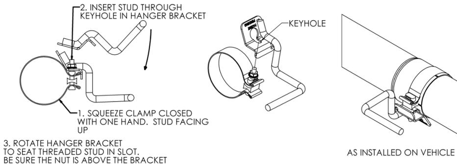
2. Using the **2.5" Clamp**, install the reduced end of the **Extension Pipe** over the factory exhaust system behind the "Y" pipe. Install the **Hang Tight™ Hanger** Clamp assembly over the Extension pipe and into the factory rubber insulator. Install the **Mid Pipe** if required using a **3.0" Clamp**, see the chart below for pipe modifications. Cut the **Extension Pipe** if required.
