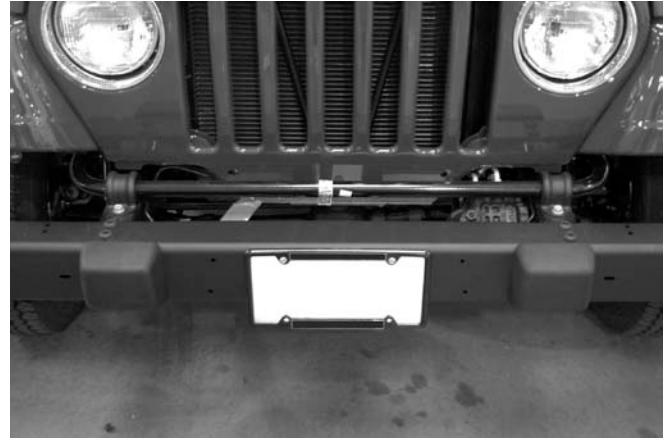
Figure #8 – Factory Front Panel Removed
