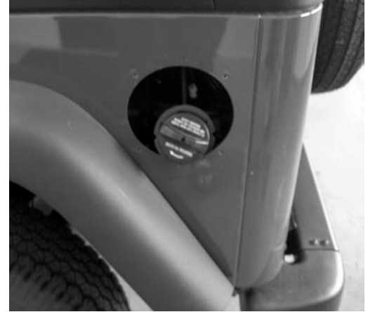
Figure #1 – Remove Gas Tank Outer Flange
