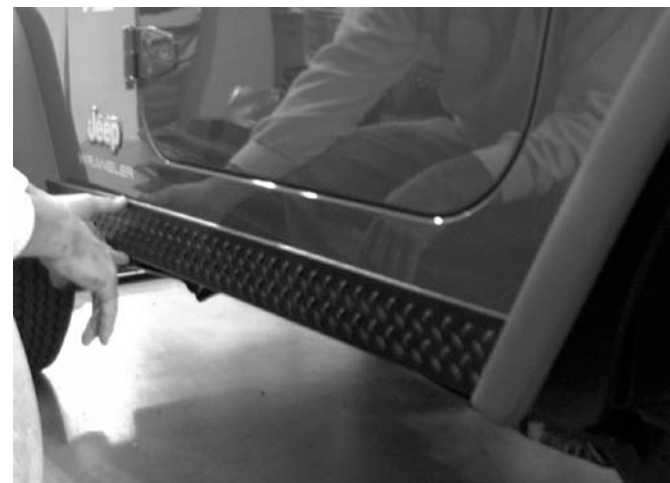
Figure #7 – Install Side Panel
