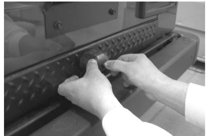
Figure #5 – Reinstall Tire Stop & Tire
