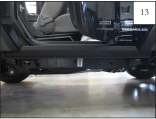
Once all tape liners are peeled, press down on entire length of part again applying 30 PSI to the taped areas. NOTE: The tape reaches maximum adhesive bond after 24 hours of contact. Do not wash vehicle for 24 hours.
