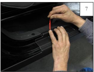
Pull 1/4" tape liner tab 2. NOTE: Refer to step 1 for additional tape tab identification.
