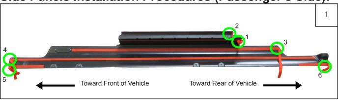
Using a marker, number the tape tabs as shown:
