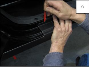
Pull 1/2" tape liner tab 1. NOTE: Take care not to catch tape liner of other pieces of tape and accidentally pull their liners off as well. NOTE: Refer to step 1 for additional tape tab identification.
