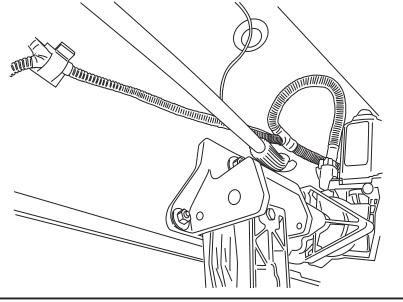
Remove driver side front kick panel and door sill plate. Roll back carpet to access hole for passing trigger wire into cab of vehicle.
