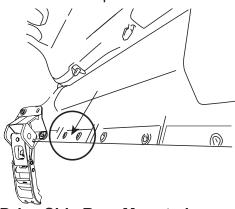
**Drive Side Rear Mounted** (In between two rivets just forward of mounting location, as shown above)
