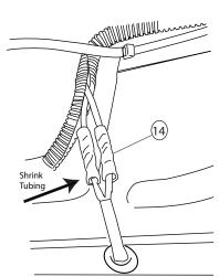
Close and wrap with conduit and electrical tape. Secure all loose wires with cable ties with lamp wires pulled upward to avoid any wire snagging.
