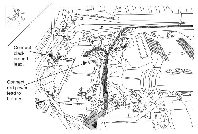
Attach wire harness (4) to controller (5) (make sure connector locking tabs fully engage). Mount controller with the two 11" tie wraps (16) to factory conduit, just forward of battery.
