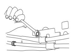
**A.** Remove bolt with 13mm box wrench or socket.
