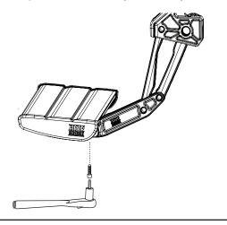
On each side of the vehicle measure from the rear linkage to end of the board. Measurement should be approximately 11" as shown below.
