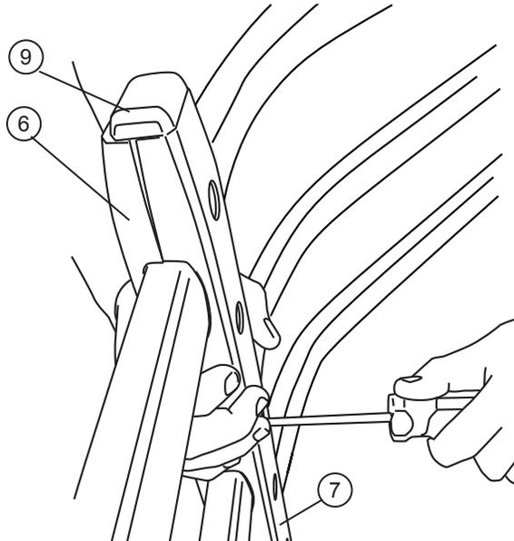
**NOTE:** Do not over tighten as this may strip out. Fastener will reach a noticeable stopping point.
