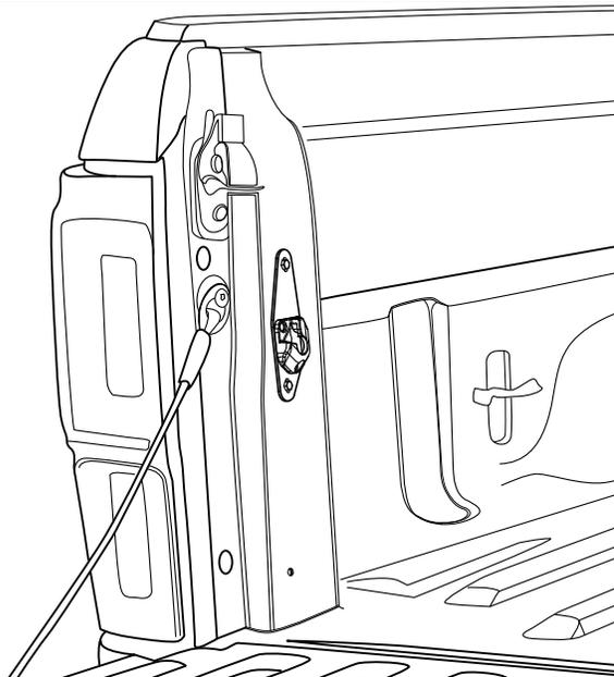
Tighten fasteners. Make sure pivot opening in bracket opens towards the rear of the vehicle.
